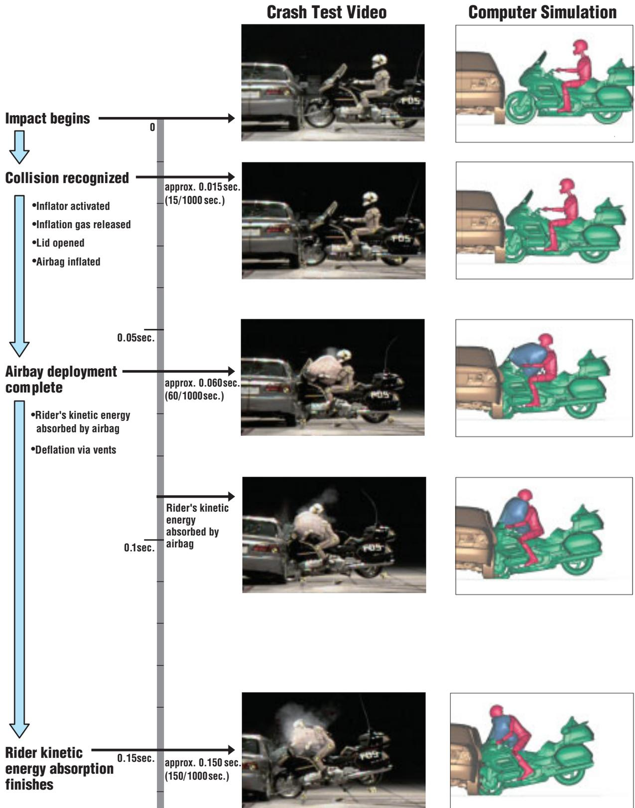
(Side collision with a stationary vehicle (Honda Accord) at 50km/h)
